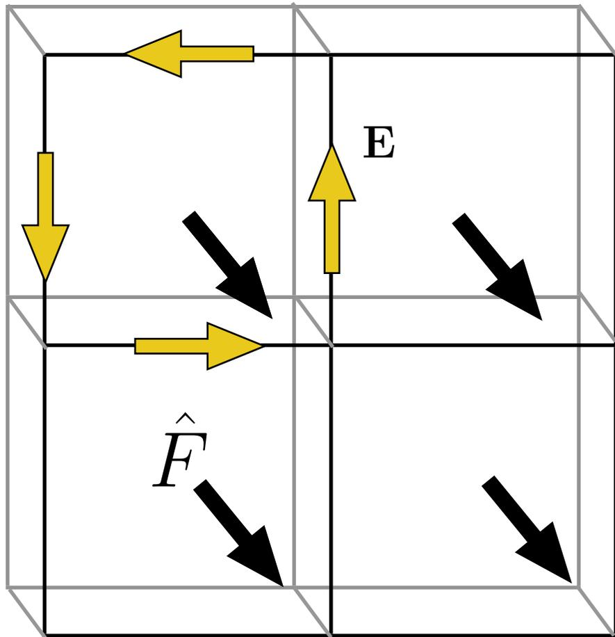
Electric Field from Fluxes from Solver
