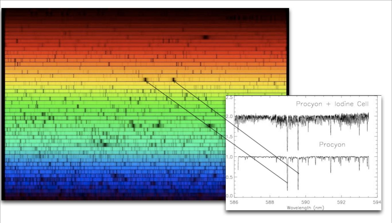
A stellar spectrum from The Keck Telescope. The velocity of the star along the line of sight is obtained by very accurately measuring the positions of the stellar absorption lines relative to a set of reference lines created by passing the light through an iodine cell which is at rest with respect to the telescope.
