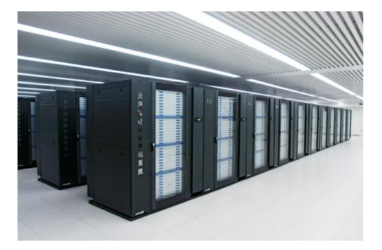
Hybrid CPU/GPU cluster (XEON/NVIDIA) 186K cores 4.7 Pflops peak speed Proprietary interconnect
