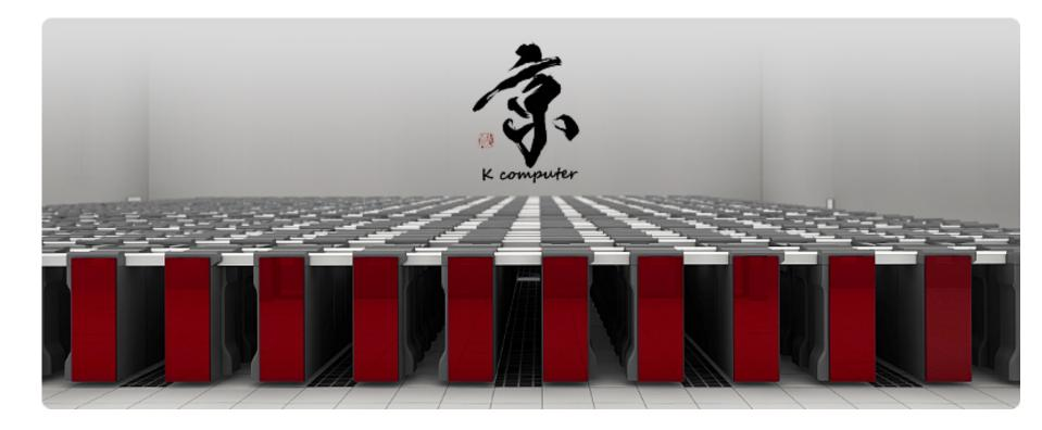
88,000 Sparc64 CPUs, 8 cores/CPU → 700K cores 11.28 Pflops peak speed Tofu interconnect (6D torus = 3D torus of 3D tori)
