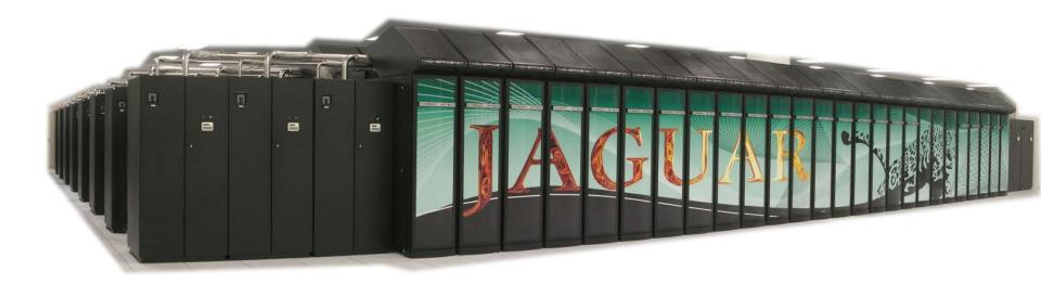
37,360 AMD Operton CPUs, 6 cores/CPU → 224K cores 2.3 Pflops peak speed 3D torus interconnect
