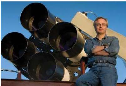
*Los Alamos National Laboratory astrophysicist Tom Vestrand poses with the fast-slew array of telescopes for RAPTOR (RAPid Telescopes for Optical Response) system. RAPTOR is an intelligent visual system that scans the skies for optical anomalies and zeroes in on them when it detects them. This unique capability allowed astronomers to witness the birth of a black hole in the constellation Leo.*
